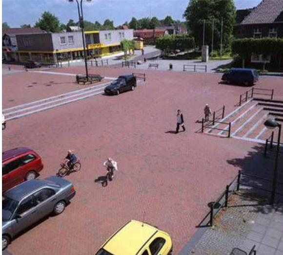
The term '*level surface*' is used to describe streets and spaces without a vertical kerb to separate the carriageway for vehicles from areas for pedestrians only. This means that the entire street is at a single level.
